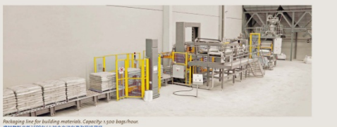
Packaging line for building materials. Capacity 1.200 bags/hour 建筑材料生产线1200包/小时全自动包装和码垛设备
